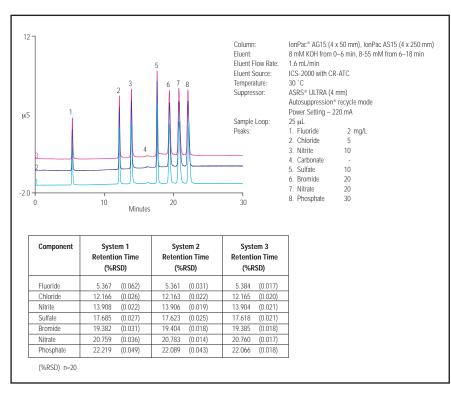
Reagent-Free IC produces consistent lab-to-lab eluent concentrations for highly reproducible retention times and peak areas. Results are the same day-to-day, system-to-system, and labors-to-labors.
